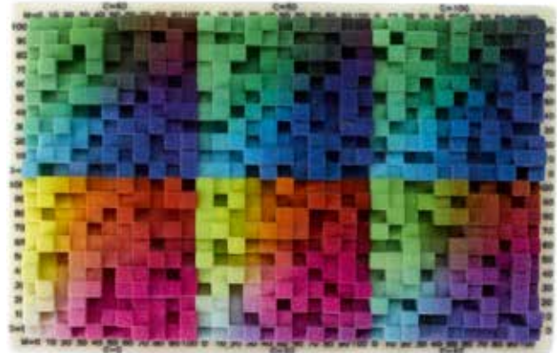
By using Cyan, Magenta, Yellow, and Black, millions of colors are possible with a full-spectrum color 3D printer.
