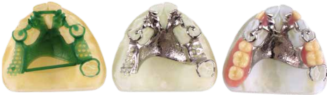
3D printing is revolutionizing dentistry. Above, a printed wax-up (prosthesis pattern) on a printed dental model, cast in metal and assembled into partial denture.
