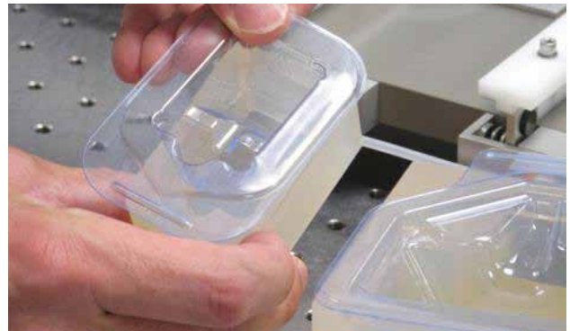
Vacuum forming can be done with 3D printed molds for pre-production or short run production.
