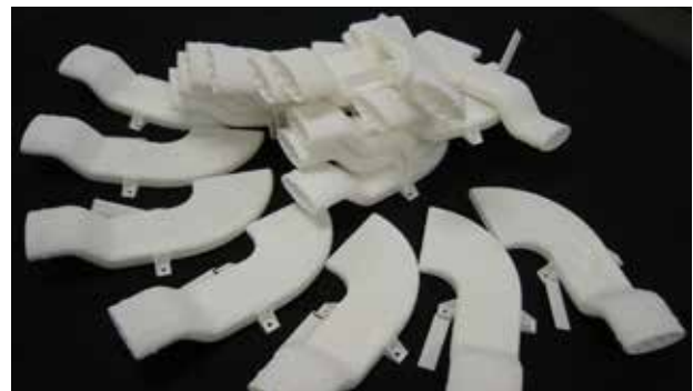
Aircraft air ducting geometry is no longer limited by the means of production so it can be printed lighter and stronger.
