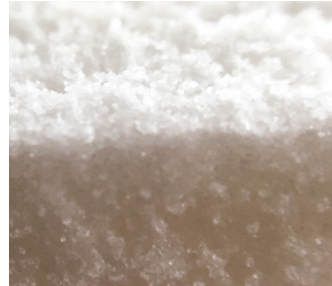
Macro view of SLS 'Orange peel' effect
